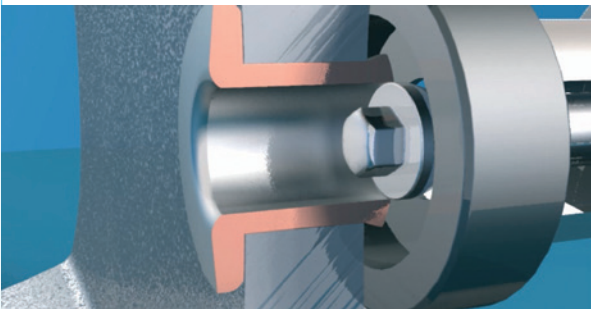
Cross section of the copper bush before and after the pressing process
