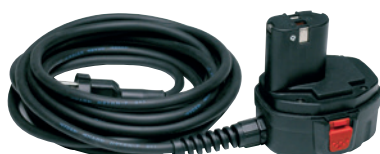
BPS230.14 Switching power supply Technical specifications: Input: 230V; 50 - 60 Hz; Output: 14.4V; Thermal protection with short circuit; Max. current: up to 5A with uniform use; 23A for 50 seconds; 30A for 8 seconds
