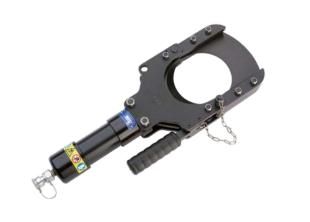
The hydraulic cutting head TC120 is suitable for cutting cables up to a maximum diameter of 120 mm. The practical snap closure allows for easy handling. The special cut and the special geometry of the cutting blades ensure a «straight cut». The tool is equipped with a quick-release, oil-loss-free coupling that allows it to be connected to a hydraulic pump with a maximum operating pressure of 700 bar.
