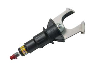
The hydraulic cutting head TC065-SC is suitable for cutting copper, aluminum and telephone cables up to a maximum diameter of 65 mm. The cutting blades are therefore made of particularly high-quality steel and heat treated to ensure a long service life. The tool is equipped with a quick-release, oil-loss-free coupling that allows it to be connected to a hydraulic pump with a maximum operating pressure of 700 bar.
