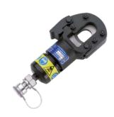
The hydraulic cutting head TC025 is suitable for cutting solid or very hard materials up to a maximum diameter of 25 mm. The cutting blades are therefore made of particularly high-quality material. The tool is equipped with a quick-release, oil-loss-free coupling that allows it to be connected to a hydraulic pump with a maximum operating pressure of 700 bar.
