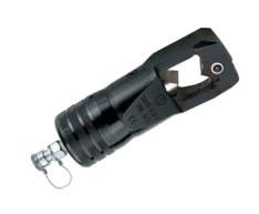
This tool is suitable for loosening square and hexagon nuts as well as fastening bushings (see table). Time-consuming and spark-causing work such as grinding or cutting is not necessary. The hydraulic nut splitter is equipped with a quick-release, oilloss-free coupling that allows it to be connected to a hydraulic pump with a maximum operating pressure of 700 bar.
