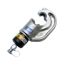
The RHC131LN hydraulic crimp die is equipped with a quick-release, oil-loss-free coupling that allows it to be connected to a hydraulic pump with a maximum operating pressure of 700 bar. With the RHC131LN the die contact gap is 42 mm. It is therefore particularly suitable for crimping larger cross-sections.
