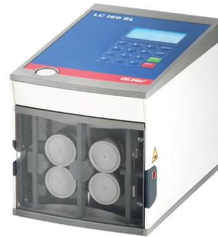
The LC 160 SL was specially developed for precise and gentle cutting to length of pneumatic, medical and many other types of tubing. Thanks to its special cutting technology with just one blade and a precise guide, the device guarantees exact 90-degree cuts of the highest quality - without deformation.
