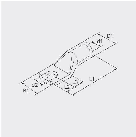
**DIMENSIONI****L1 (mm):** 59.5**L2 (mm):** 14.5**L3 (mm):** 14.5**B1 (mm):** 23.0**d1 (Ø):** 10.0**d2 (Ø):** 15.0**D1 (Ø):** 14**NOTA**
