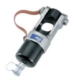
The ECW-H3D hydraulic crimp die is equipped with a quick-release, oil-loss-free coupling that allows it to be connected to a hydraulic pump with a maximum operating pressure of 700 bar (see Hydraulic Pumps, page 146). The crimp dies correspond to the size 3 as per DIN 48083. With the adapter AU230-130D all crimp dies of the 130 kN tools can be used.
