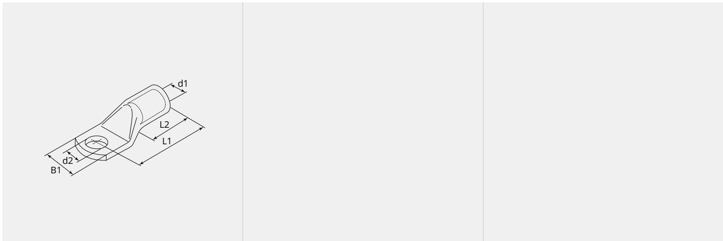
**DIMENSIONI****L1 (mm):** 24.0**L2 (mm):** 10.0**B1 (mm):** 8.5 **$d_1 (\varnothing)$ :** 3.8 **$d_2 (\varnothing)$ :** 5.3**NOTA**
