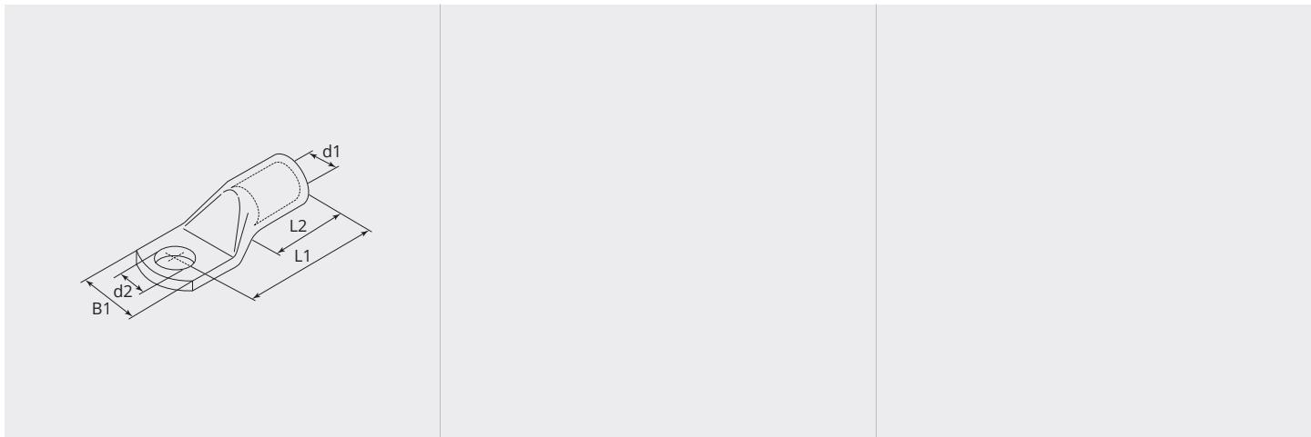
**DIMENSIONI****L1 (mm):** 117.0**L2 (mm):** 70.0**B1 (mm):** 55.0**d1 ( $\varnothing$ ):** 27.5**d2 ( $\varnothing$ ):** 13.0**NOTA**
