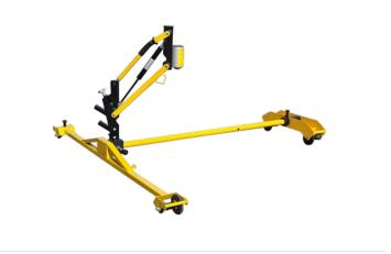
The support mechanism, which secures the portable timber sleeper drilling machines and the portable impact wrech, incorporates a gas pressure spring to give a constant, balanced control to the machine during operation. Fitted with insulated wheels, the trolley does not interfere with the track electrical circuits. The trolley is easily closed and can comfortably be carried by a single operator.
