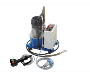
The 220V electric hydraulic pump CPE-1 operates with a single-phase motor and a maximum operating pressure of 700 bar. The pump is controlled via a hand-held remote control. By pressing a certain button on the pump at any time the pressure can be reduced. There is also a version for 110V available. Both versions have protection rating of IP55.
