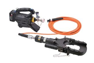
It is not always possible to identify a cable to be worked on with absolute certainty. Therefore, the clear determination of the absence of voltage sometimes causes major difficulties. In order to protect the workers from danger, safety cutting systems are used to determine the absence of voltage in accordance with DIN VDE0105 T.1, Section 9.6.4 (07 83).
