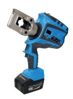
The BA500 hydraulic battery-powered tool is suitable for installing electrical crimp connections on cables up to 300 mm². This crimping tool uses standard 50 kN crimping dies that are compatible with other tools and heads.
