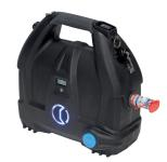
The hydraulic battery pump B70M-P36 has a 36V - 8.0 Ah battery and operates with an operating pressure of 700 bar. The pump can be operated with a hand of foot pedal remote control. They are equipped with a manual button for operation and pressure relief (electronically locked for safety reasons when the hand remote control is used). With just one battery charge up to 90 cuts AE-KEBY 3 x 150 mm can be performed.
