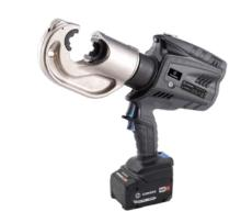
The hydraulic crimper B1350L-C is equipped with a double piston hydraulic. The 180 ° rotatable head allows easy handling even in narrow and confined spaces. The contact gap of the head is 42 mm and is especially suitable for crimping large cross-sections.
