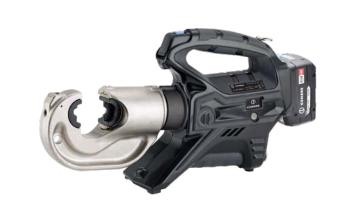
The hydraulic crimper B1300L-C is equipped with a double piston hydraulic. The 180° rotatable head allows easy handling even in narrow and confined spaces. The contact gap of the head is 42 mm and is especially suitable for crimping large cross-sections.
