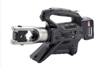
The hydraulic crimper B1300-UC is equipped with a double piston hydraulic. The 180° rotatable head allows easy handling even in narrow and confined spaces. A chip controls the operation and automatically shuts off the motor as soon as the crimping has completed. This saves energy and increases the service life of the battery.
