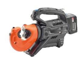
The insulated hydraulic crimp B1300-C-KV is equipped with a double piston hydraulic. The crimp die can be rotated through 180°, which makes it possible to use possible in a confined space. A chip controls the operation and automatically shuts off the motor as soon as the crimping has completed. This saves energy and increases the service life of the battery.
