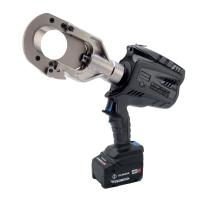
The hydraulic battery-operated cutter B-TC650 with double piston hydraulic was developed for cutting copper, aluminum and telephone cables up to a maximum diameter of 65 mm. Because of the snap closure on the head, the tool can also be used to cut endless material. The good handling is guaranteed by the 335° rotatable head.
