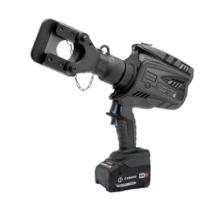
The hydraulic battery-operated cutter B-TC450 with double piston hydraulic is especially suitable for cutting solid or very hard materials up to a maximum diameter of 45 mm. Because of the snap closure on the cut- ting head, the tool can also be used to cut endless material. The handling is guaranteed by the 180° rotatable head.
