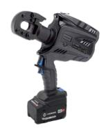
The hydraulic battery-operated cutter B-TC250 is suitable for cutting solid or very hard materials up to a maximum diameter of 25 mm. The cutting blades are therefore made of particularly high-quality material. The 180° rotatable head and the practical snap closure allow easy handling. The tool has a double piston hydraulic quick-feed. Due to its characteristics, this tool is often used for overhead lines.
