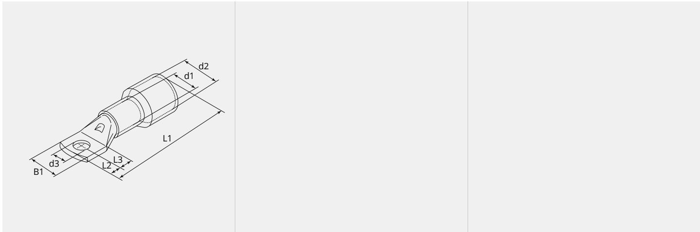
**DIMENSIONI****L1 (mm):** 55.0**L2 (mm):** 8.0**L3 (mm):** 9.0**B1 (mm):** 19.0**d1 (Ø):** 10.0**d2 (Ø):** 13.8**d3 (Ø):** 8.4**NOTA**
