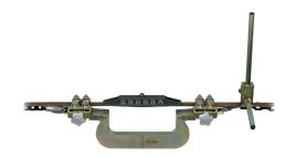
Installation is much easier with the AD-GW tool, and the time required to fit overhead line joint clamps on grooved contact wires is reduced. The tool is integrated in the existing hoist with its overhead line tensioning clamps.
